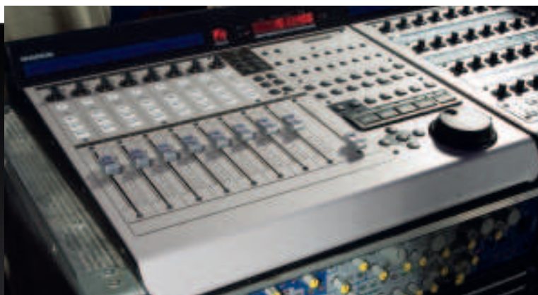
▲ We'll be using the Mackie Control Universal Pro for total hands-on mix control
