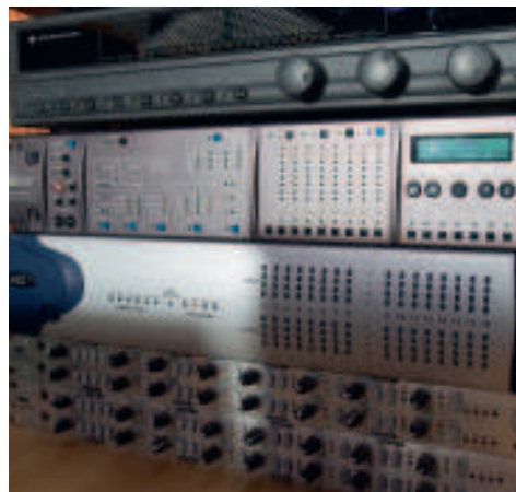
▲ The quality of the A/D conversion won't be an issue with either of our mixes today – we're using the acclaimed Prism ADA8 for both
